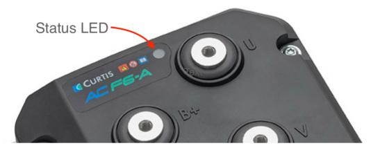
In the absence of a Curtis programmer, the Motor Controller status can be obtained by checking the status indicator on the controller per the illustration above. The status indicator is a translucent window on the cover, which blinks red and yellow LEDs whose meanings are:
