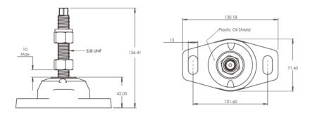
Dimensions (in mm) of supplied motor mounts with 5/8" stud.
