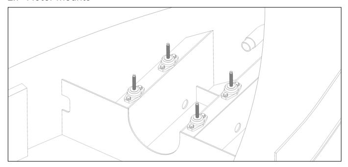
Check that measurements are in accordance with the drawings provided: Motor mounts need to be fixed with 10mm stainless steel bolts and locking nuts. Loosely fit to allow for motor and shaft alignments later. Refer to the Törkmar Motor Mount technical drawings for the required mount layout.
