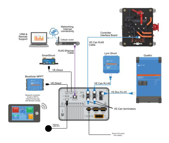
Note that the BMS cable type is dependent on the installed battery or Battery Management System. Victron has a guide to which cable to use which can be found at:
